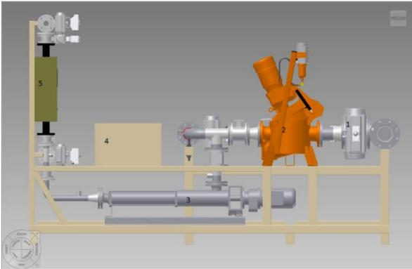
The schematic 3D model of the pre-treatment line with the substrate flow from right to the left. The green box is the treatment chamber where the electrical pulses is applied to the substrate.
