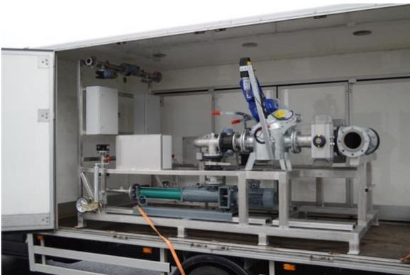
The pre-treatment line at delivery from the subcontractor. This unit is later mounted with all electronics and then installed in the container.
